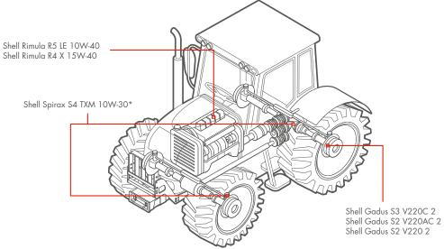
\*Shell Spirax S4 TXM is a universal tractor transmission oil (UTTO) that can also be used for hydraulic and immersed wet brake systems.
